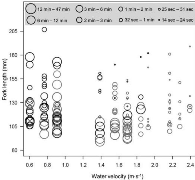
FIGURE 2. Duration (circle size) and culvert side (black = right; grey = left) of successfully passing fish by fork length and trial velocity. For fish exhibiting multiple passes, duration was averaged across all successful passages. If fish with multiple passes used the middle or right side of the pipe during at least one ascent, the resulting data point was chosen to reflect this with a black circle.
