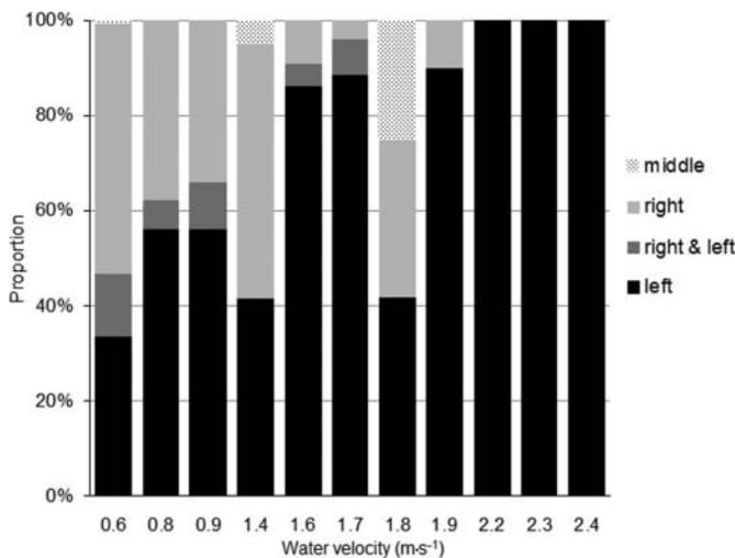
FIGURE 3. Proportion of fish choosing the middle, the right, the right and left, and only the left sides of the culvert during passage trials.
