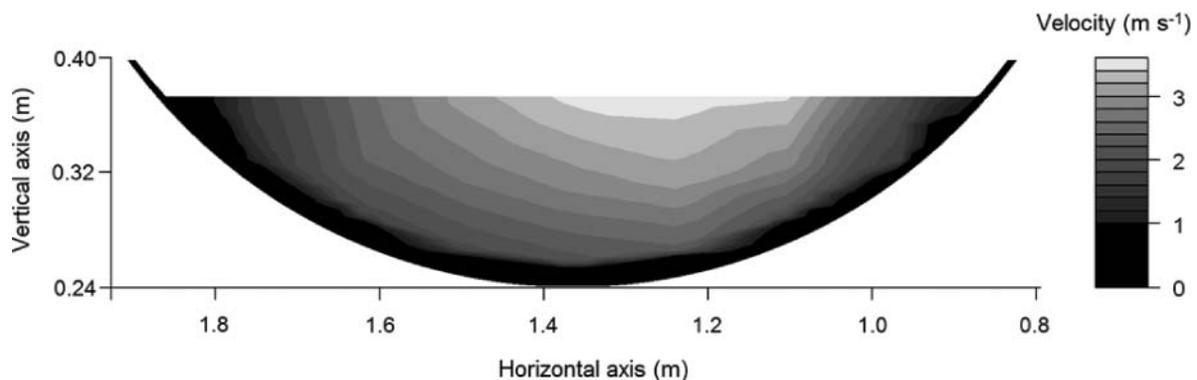
FIGURE 1. Velocity contour profile at a modeled average velocity of 2.4 m/s ( $Q = 0.34$  m<sup>3</sup>/s; slope = 8.6%) at the center of the culvert looking downstream; the vertical axis is exaggerated to provide greater resolution of the variation in velocities.
