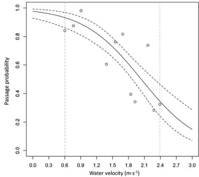
FIGURE 4. Fitted logistic regression curve (solid line) giving average culvert passage probabilities for various target velocity values and pointwise 95% lower and upper confidence bands (dashed lines).
